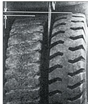
In no case should a difference in diameters be corrected by adjusting inflation pressure.
